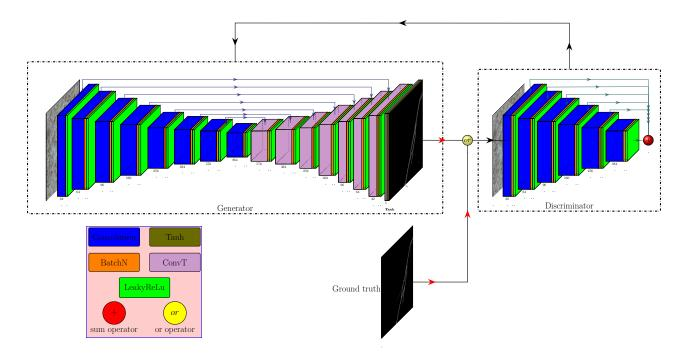
Figure 1. Proposed conditional GAN architecture and methodology. The network has one Generator and one Discriminator sub-networks. The input of the Discriminator is the output of Generator combined with the input image. As training progresses, the Generator produces segmented images resembling more and more to the ground truth. The Discriminator then learns to discriminate between the ground truth image and the images produced by the Generator.
