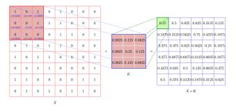
Figure 2. Example of a convolution of an image X with a Gaussian blur kernel (or filter) K. X with size  $8 \times 8$  passes through a convolution kernel function K with size  $3 \times 3$ . The filter moves toward the right part of the image and new pixel values are computed. The sliding window (stride) is of 1 pixel.
