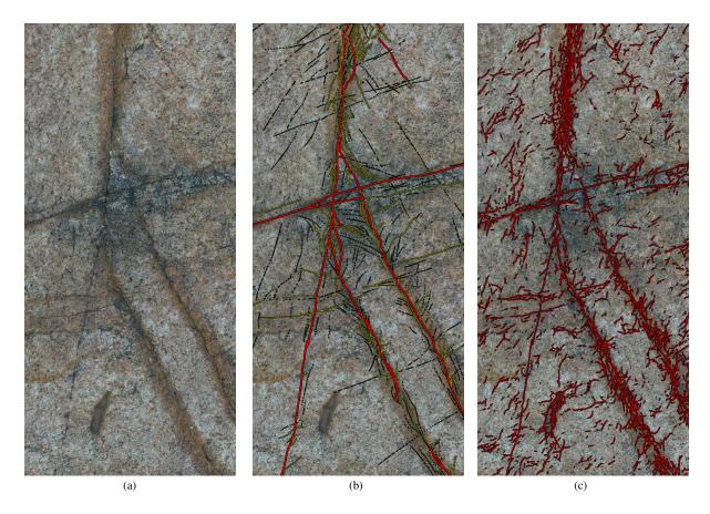
Figure 4. An image patch,  $1800 \times 840$ , taken from the test region (a), the corresponding annotation made by human expert (major faults in red, more minor faults in yellow, and uncertain faults in black) (b) and our CGAN (c) prediction.
