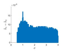
Fig. 2: Trade-off between coupling strength  $\sigma$  and maximum sampling interval  $\bar{h}_1 = \bar{h}_2$ , for the system (40), with  $\alpha = 0.01$ .
