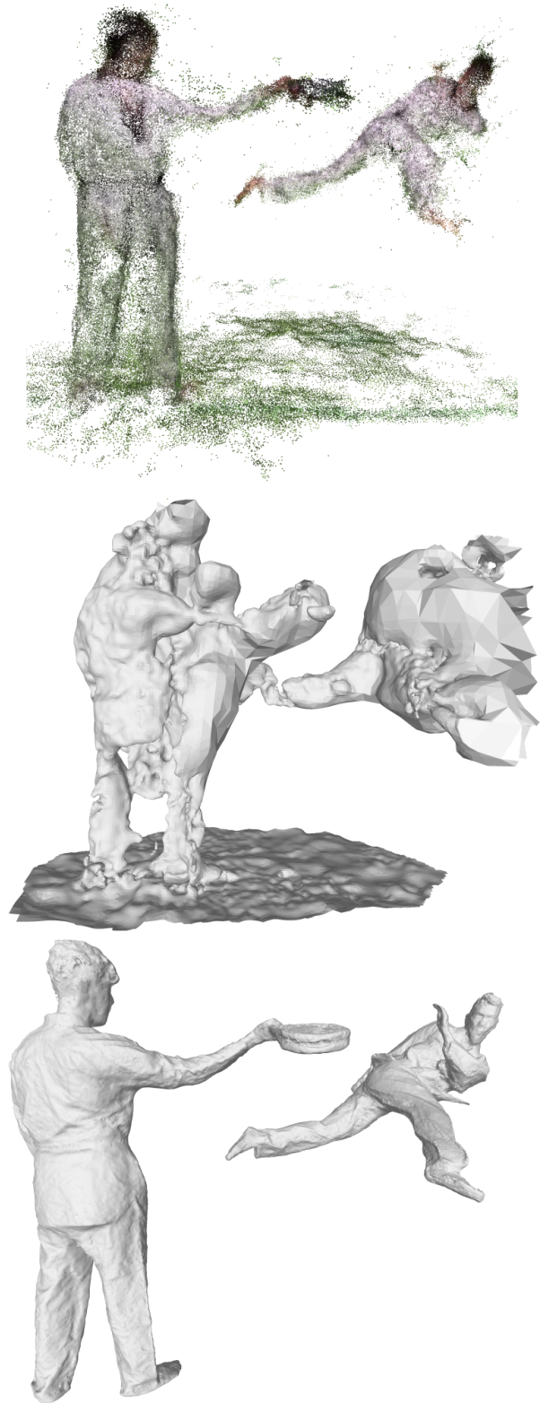
Fig. 18 ( top ) Results provided by [8] on the kick 540 sequence. ( middle ) Poisson Reconstruction of the output point cloud of [8]. ( bottom ) Our result.
