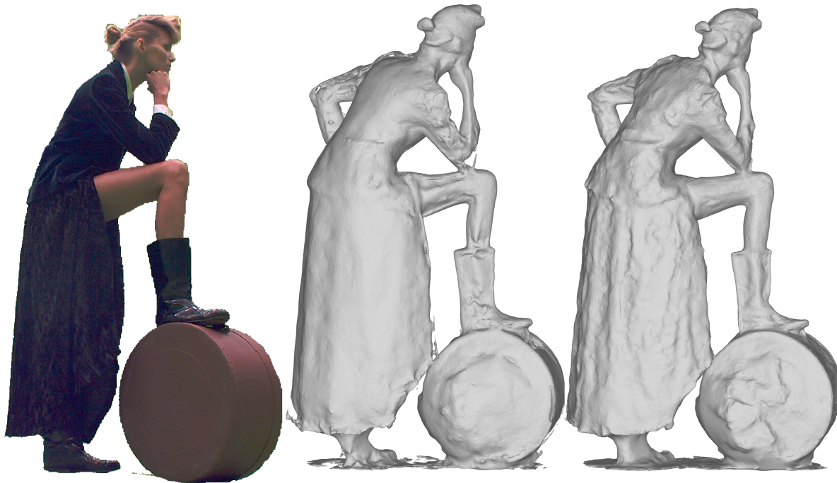
Fig. 1 Challenging scene captured with a passive RGB multi-camera setup [9]. ( left ) one input image, ( center ) reconstructions obtained with classical 2D features [10], ( right ) proposed solution. Our results validate the key improvement of a CNN-learned disparity to MVS for performance capture scenarios. Results particularly improve in noisy, very low contrast and low textured regions such as the arm, the leg or even the black skirt folds, which can be better seen in a brightened version of the picture in Figure 17.
