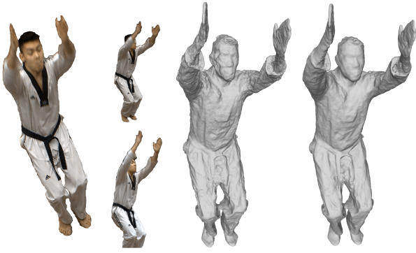
Fig. 12 (Left) 3 input images, (middle) plane based classifier, (right) volumetric classifier. The face is highly occluded in many views (left) making the reconstruction noisy and inaccurate when using a planar support whereas the volume counterpart yields smoother and more accurate details.
