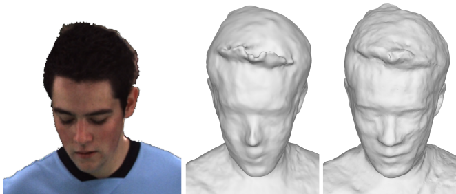
Fig. 21 Close up of the face of the subject from [23] ( left ). The reconstruction provided by the authors ( middle ) is very smooth compared to our result ( right ).
