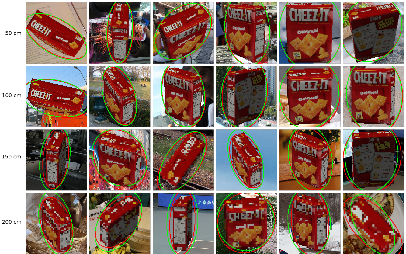
Figure 4. Predicted ellipses (green) for more distant camera positions (indicated on the left). Ground truth ellipses are in red. All the images have the same size because only the rescaled crop around the object is passed to the network. The bottom images would appear much smaller in the original full-size images.
