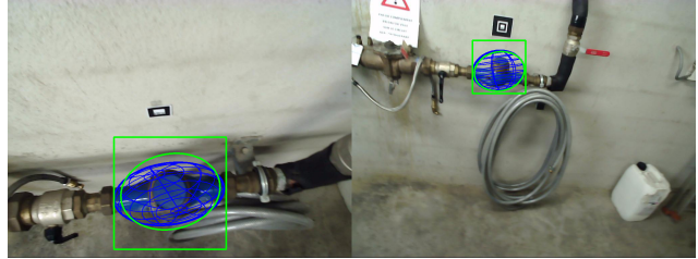
Figure 10. Predicted ellipses and ground truth projections of the ellipsoid in WatchPose.
