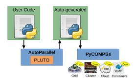
Figure 3. Overview of the AutoParallel Module.
