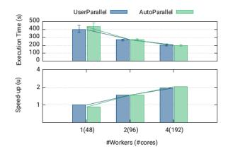
**Figure 5.** Cholesky: Execution times and speed-up with respect to the *userparallel* version using a single worker (48 cores).
