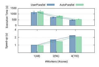
**Figure 8.** QR: Execution times and speed-up with respect to the *userparallel* version using a single worker (48 cores).
