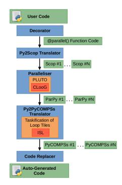
Figure 4. Internals of the AutoParallel Module.
