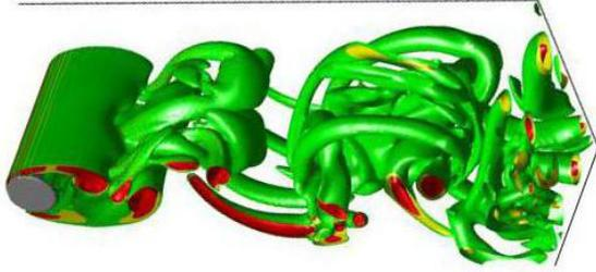
Figure 1: Q-criterion – 13 vortex shedding cycles after the learning period – from the 3D DNS at Reynolds 300.
