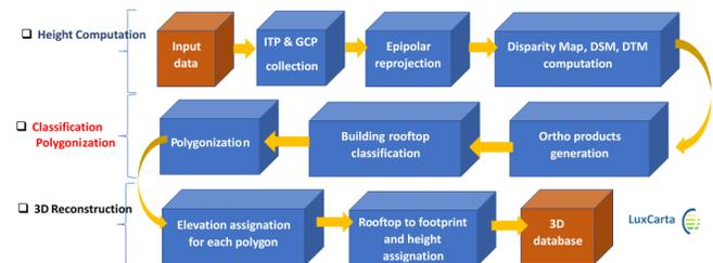
Fig. 1: Proposed pipeline.
