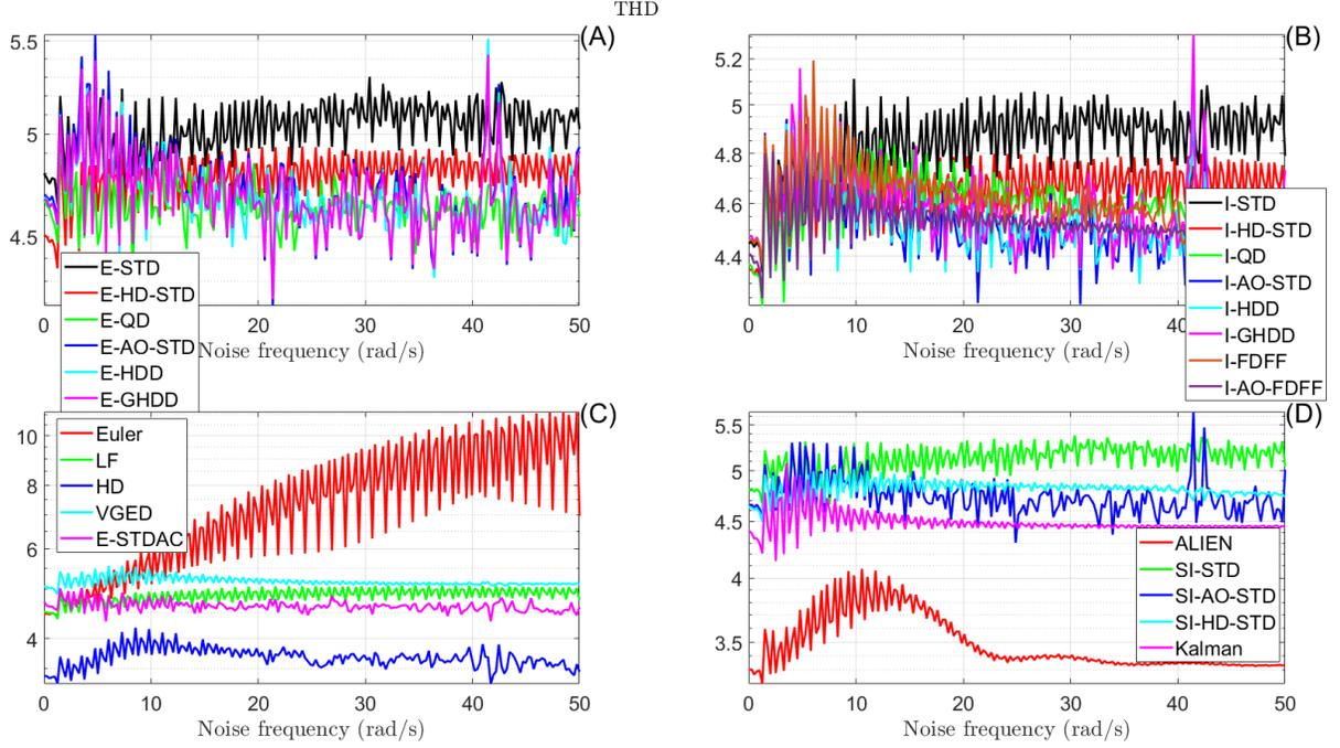
Figure 31: THD for the first-order differentiation concerning noise frequency. Input noise:  $0.05\sin(\omega t)$ ,  $\omega$  is the noise frequency. Parameters are shown in Table 6 ( $h = 50\text{ms}$ ).
