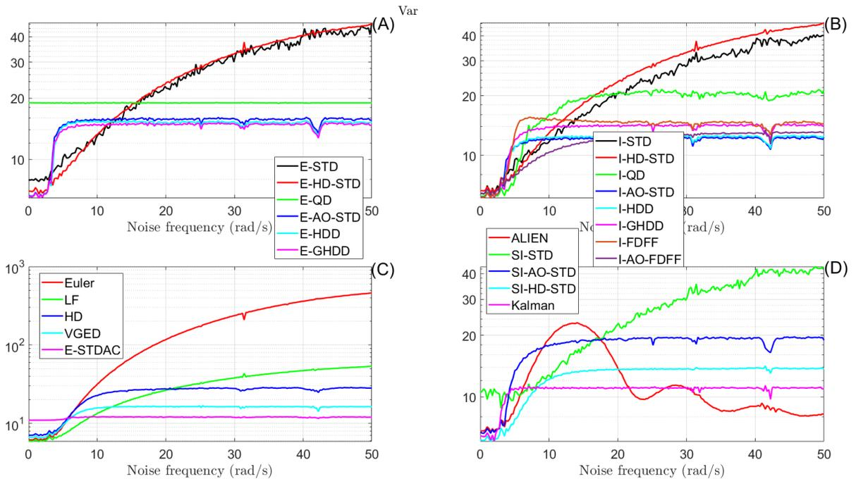
Figure 30: Variation for the first-order differentiation with respect to noise frequency. Input noise:  $0.05\sin(\omega t)$ ,  $\omega$  is the noise frequency. Parameters are shown in Table 6 ( $h = 50\text{ms}$ ).
