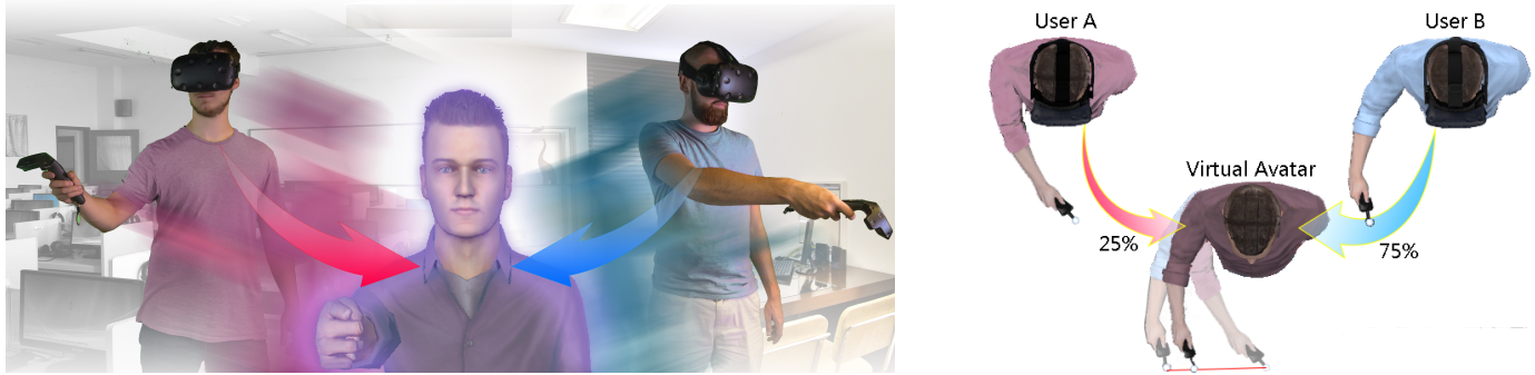
Fig. 1. Our “Virtual Co-Embodiment” experience enables a pair of users to be embodied simultaneously in the same virtual avatar (Left). The positions and orientations of the two users are applied to the virtual body of the avatar based on a weighted average, e.g., “User A” with 25% control and “User B” with 75% control over the virtual body (Right).
