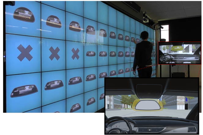
Figure 4. Usability study setup: the target shape is displayed with a transparent yellow color in a realistic environment on an external screen next to the wall-sized display.
