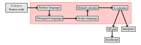
Fig. 2 High-level architecture of the CATALA compiler (red box)
