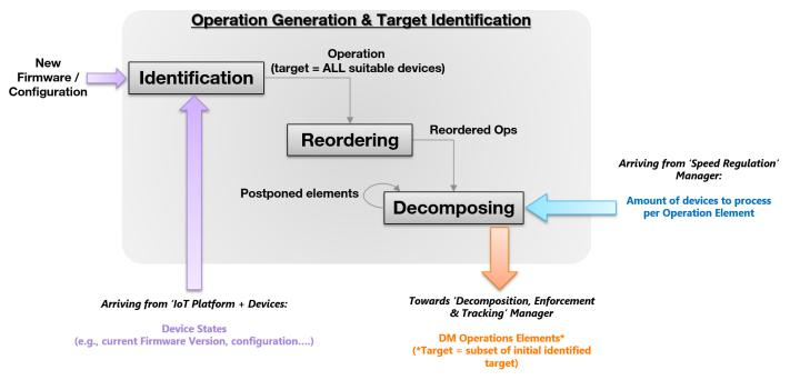
Figure 3. Operation Generation & Target Identification autonomic workflow
