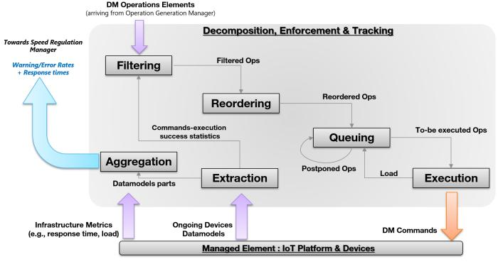
Figure 2. Decomposition, Enforcement & Tracking autonomic workflow
