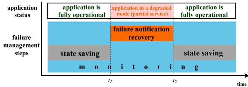
Figure 4: Failure Management Steps of an Applicative Entity
