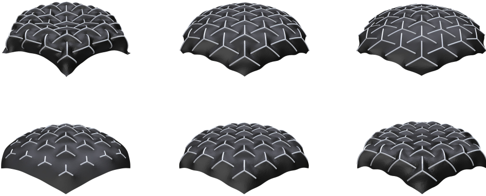
Figure 8: We show the effect of two design parameters on the equilibrium shape of the star metamaterial: the length of the star arms \ell and their thickness h . For this experiment we print 37 stars on a hexagon of fabric with side length 67 mm. In the top row we fixed \ell = 10 mm and set, from left to right, h with a decreasing radial gradient from 0.6 mm to 0.2 mm, a constant value of 0.4 mm and an increasing gradient from 0.2 to 0.6 mm. In the bottom row we fix h = 0.3 mm and prescribe three different radial gradients for \ell : a decreasing gradient from 10 mm to 4 mm, and constant value of 7 mm and an increasing gradient from 4 mm to 10 mm.
