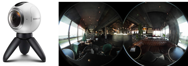
Fig. 1: (Left) Samsung Gear 360 Camera. (Right) Gear 360 dual-fisheye output image (3840 × 1920 pixels).
