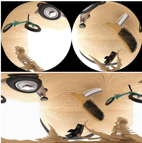
Fig. 4: Example of a synthetic scene captured with a 360° fish-eye camera model: (top) original spherical image, (bottom) stitched equirectangular image.
