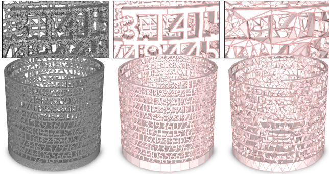
Fig. 10. Reconstruction of TOWER OF PI. 10.8K planar shapes are detected from 2.9M input points (left) and assembled by our algorithm into a concise polygonal mesh of 12.1K facets (middle). Each digit is nicely represented by a few facets (see closeups). In contrast, the mesh produced by the traditional approximation pipeline (Screened Poisson [Kazhdan and Hoppe 2013] then QEM edge collapse [Garland and Heckbert 1997]) at the same output complexity fails to preserve the structure of the digits (right).
