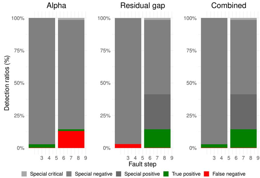
Figure 4.5: Comparison of the detection success of the alpha and residual gap based methodologies, and their combination for persistent bit-flips in the matrix-vector product or preconditioner ( $p_i$  or  $r_{i+1}$ .) steps of PCG.
