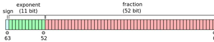
Figure 2.1: IEEE 754 double-precision binary floating-point format.
