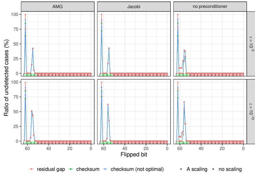
Figure 4.2: Detection performance of residual gap deviation and checksum-based methodologies for soft errors in the matrix-vector calculation with persistent faults in  $p_i$  for the matrix-vector product.
