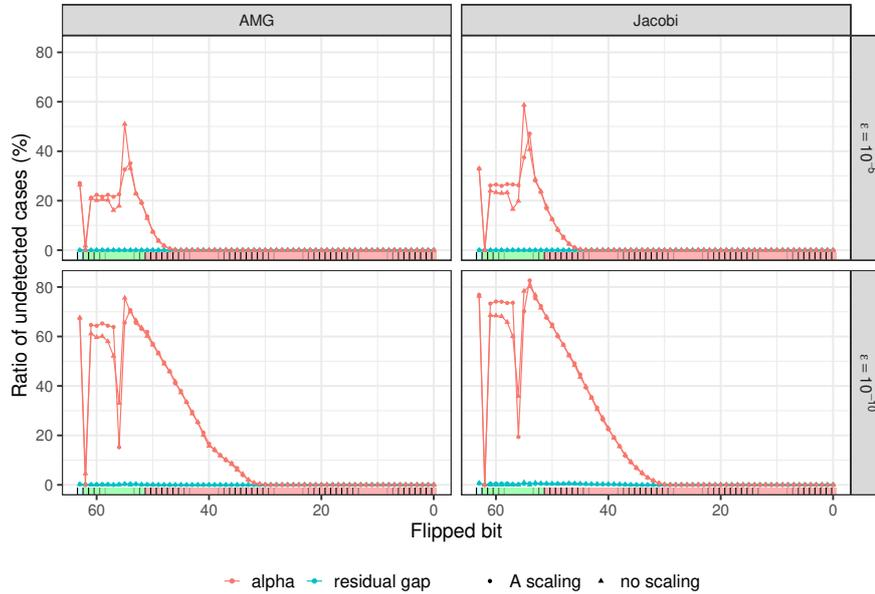
Figure 4.4: Detection performance of the residual gap and  $\alpha$ -based methodologies for soft errors in the preconditioner calculation with persistent faults in  $r_{i+1}$  in the preconditioner calculation.
