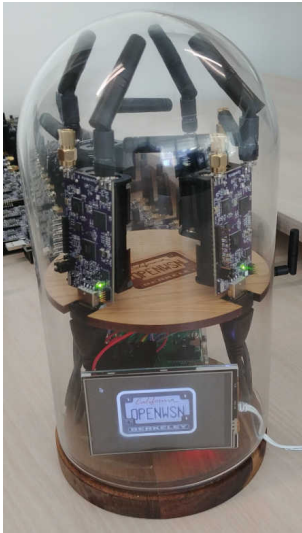
Fig. 11. We reuse the OTBox from the OpenTestbed [26] to serve as a QuickCal Box.
