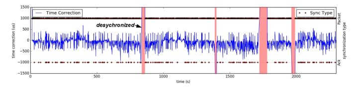
Fig. 17. Time correction of  $SC\mu M$  against an OpenMote while they form a heterogeneous 6TiSCH network. We use the OpenWSN implementation, which we have ported to the  $SC\mu M$  chip.  $SC\mu M$  de-synchronized 4 times during the experiment but re-synchronized quickly.
