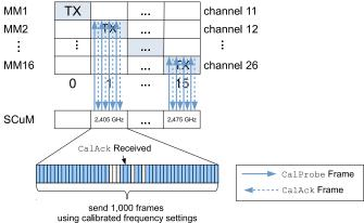
Fig. 15.  $SC\mu M$  sends 1,000 CalProbe frames and listens for CalAck frames on each of the 16 frequency channels. We define the packet delivery ratio (PDR) as the portion of CalAck frames received and use it to quantify the quality of the QuickCal self-calibration routine.
