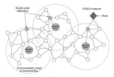
Fig. 9. Several QuickCal Box's are placed in the deployment area of the  $SC\mu M$  chip, such that each  $SC\mu M$  chip is within communication range of at least one QuickCal Box.  $SC\mu M$  uses a QuickCal Box as a reference to self-calibrate.
