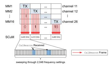
Fig. 13. QuickCal Step 1: receiving from the QuickCal Box.  $SC\mu M$  sweeps is frequency settings while listening for CalBeacon frames sent on all 16 frequencies by the OpenMote devices in the QuickCal Box. OpenMote MM1 sends CalBeacon frames on channel 11 in slot 0, OpenMote MM2 sends CalBeacon frames on channel 12 in slot 1, etc. The  $SC\mu M$  chip receives beacons at multiple frequency settings; it uses the algorithm in Section IV-C3 to determine the best setting.
