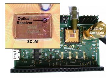
Fig. 1. Development environment of the Single Chip Micro Mote ( $SC\mu M$ ), a  $2\times3\times0.3$  mm<sup>3</sup> crystal-free mote-on-chip, which features an ARM Cortex-M0, an IEEE802.15.4 radio operating at 2.4 GHz, and an optical receiver for programming [12]. Once the firmware is loaded onto the  $SC\mu M$  chip, the chip can then be removed from its development board; all it needs to operate are a power source and an antenna.
