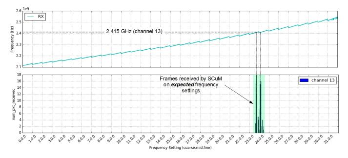
Fig. 8. Results of RX calibration (OpenMote $\rightarrow$ SC $\mu$ M) on channel 13. The top plot shows the frequency SC $\mu$ M receives on. The bottom plot is a histogram of the number of frames received by SC $\mu$ M for each frequency setting.
