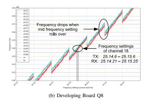
Fig. 4. Frequency of the LC oscillator as a function of the frequency setting in the range from 22.0.0 to 29.31.31 on  $SC\mu M$  development boards Q3 and Q8.
