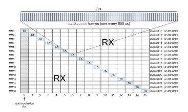
Fig. 12. The QuickCal Box schedule. Each OpenMote (numbered MM1–MM16) is assigned a different frequency channel. One after the other, each OpenMote sends 1,000 CalBeacon frames, one every 600  $\mu$ s. Slot 0 is used by MM2–MM16 to synchronize to MM1 by listening to its CalBeacon frames. Whenever an OpenMote does not transmit CalBeacon frames, it listens for CalProbe frames, to which it answers with a CalAck frame.
