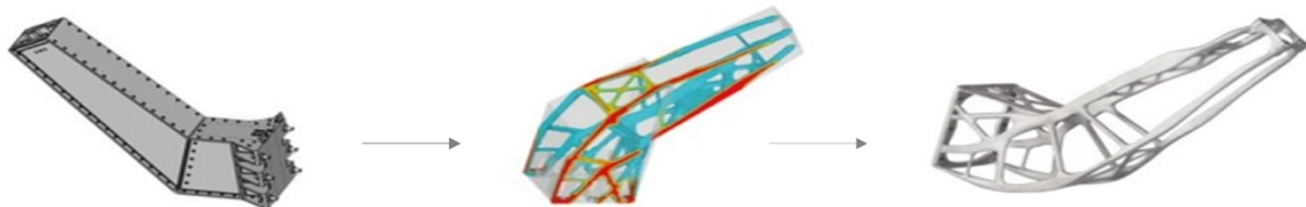
Fig. 1. Antenna bracket. Advances in topological optimization and additive manufacturing yield increasingly complex shapes with reduced weight. Left: original design. Middle: topological optimization. Right: new design.
