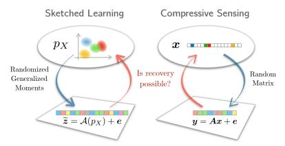
Fig. 5: The analogy between sketched learning, which uses the dimensionality reducing linear measurement  $\mathcal{A}(p_X) = \mathbb{E}[\Phi(X)]$  of a distribution  $p_X$ , and compressive sensing, which uses the dimensionality reducing linear measurement Ax of a signal x.
