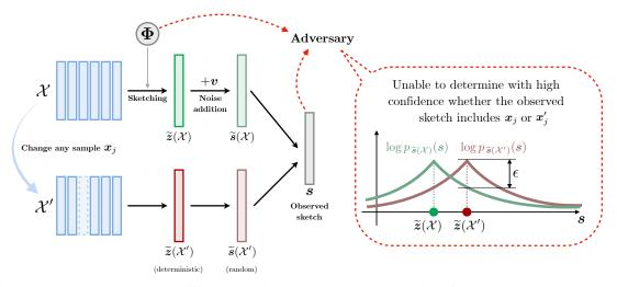
Fig. 14: When sketching with differential privacy, the output log-density of the sketch s remains close when changing one sample in the dataset (since (49) is equivalent to  $|\log(p_{\tilde{s}(\mathcal{X})}(s)) - \log(p_{\tilde{s}(\mathcal{X}')}(s))| \le \epsilon$  for all possible s). An adversary with knowledge of  $\Phi(\cdot)$  and s—as symbolized by the red arrows—could then hardly decide whether a given sample  $x_i$  was used to compute the sketch or not.
