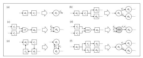
**Fig. 1.** Building blocks of a CECA diagram and their counterparts in a state machine model [7]: regular action-condition segment (a), action-condition segment with a common cause (b), OR operator (c) and AND operator (d). Additional building blocks: feedback connection (e) and branching to multiple next states with different conditions (f). Concatenation of symbols denotes logical AND. Loopback edges have been omitted for clarity.
