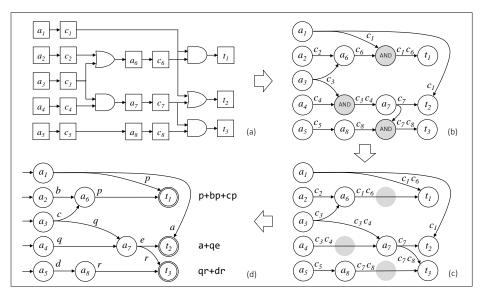
**Fig. 6.** Sample CECA diagram (a) and equivalent state machine diagram (b) as described in [7]. The same diagram with removed AND-states introduced during conversion (c) and transformed into form usable for linguistic approach (d). States representing target disadvantages are annotated with respective regular expressions.
