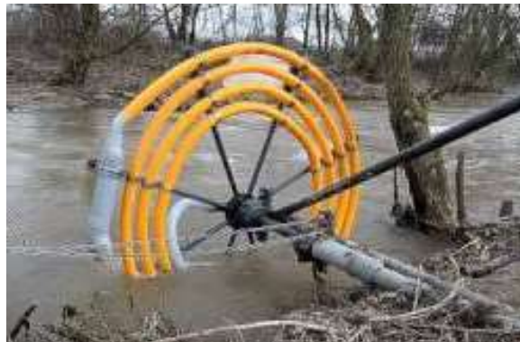
Fig. 6. Water wheel pumps
