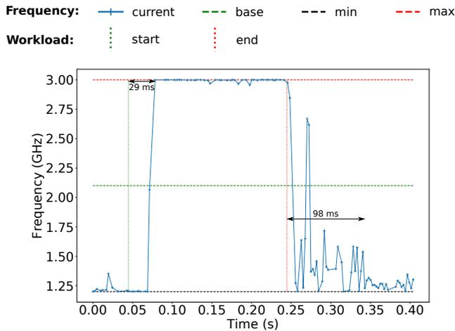
Figure 3: FTL for the Xeon E7-8870 v4 CPU.
