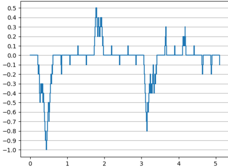
(a) Approximation process of a Brownian motion on the time interval [0, 5] with a sticky point at 0 of stickiness \rho = 4.0 using a uniform grid \mathbf{g} with step size h = 0.1
