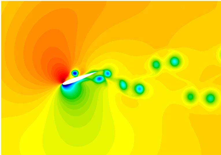
Figure 16: Pitching airfoil, laminar flow, density field
