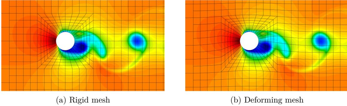
Figure 11: Comparison of movement laws, density fields,  $p=5$ , intermediate mesh
