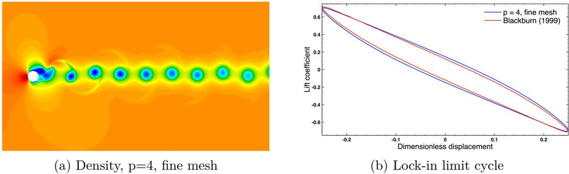
Figure 10: Numerical solution of the oscillating cylinder test case
