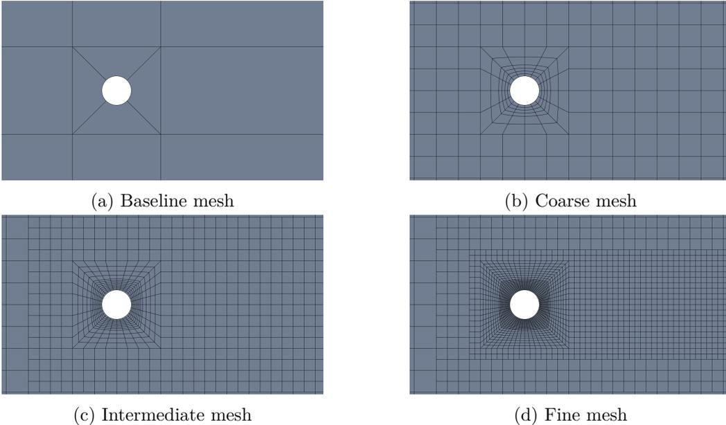
Figure 8: Different refinement levels for the cylinder simulation
