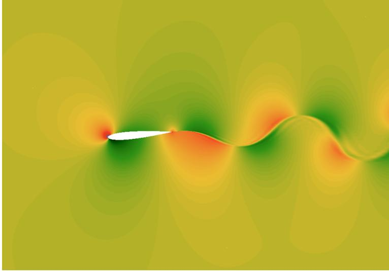
Figure 14: Pitching airfoil, inviscid flow, streamwise momentum field
