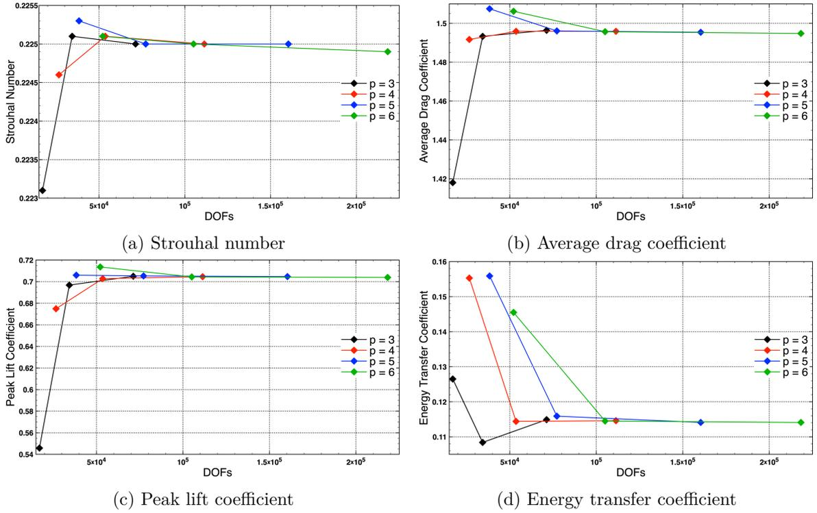
Figure 9: Oscillating cylinder flow, convergence study
