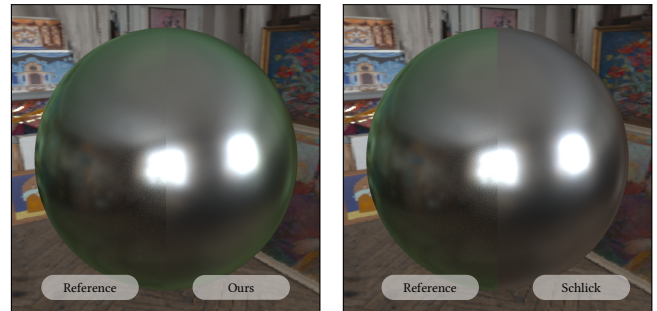
Figure 2: Our method reproduces better the edgetint than Schlick's decomposition compared to a Monte-Carlo reference. We used r = [0.44, 0.44, 0.44] , g = [0, 1, 0] and \alpha = 0.08 .
