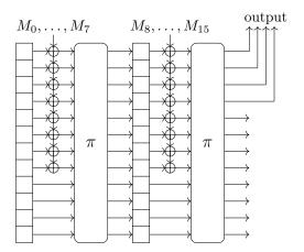
Figure 1: Sponge construction with inner permutation  $\pi$ , internal state with t=12 words and capacity c=4.
