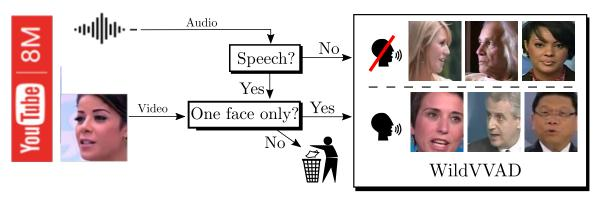
Fig. 2: Face detection and audio voice activity detection (A-VAD) are applied to each video sequence. Speaking faces are generated whenever A-VAD detects speech in conjunction with a single face. Silent faces are generated whenever A-VAD does not detect any speech.
