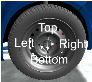
Fig. 3: The pattern to follow (it can be symmetrically reversed, and started from any nut)
