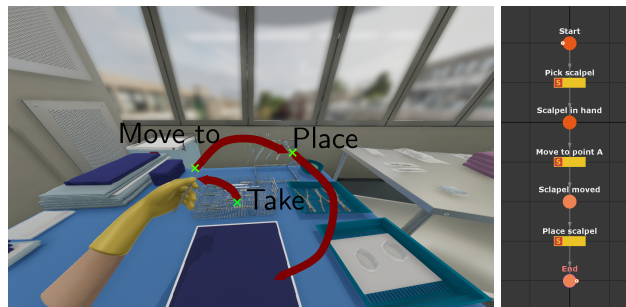
Fig. 2. The actions recorder for a pick and place task, and the corresponding scenario
