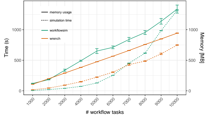
Figure 8: Average simulation time (in seconds, left vertical axis) and memory usage (maximum resident set size, right vertical axis) in MiB vs. workflow size.
