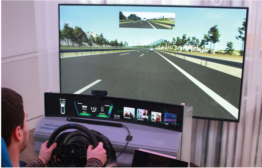
Fig. 6. Publicly deployed medium fidelity driving simulation showing a participant experiencing the concept Gamification , displayed above the steering wheel.
