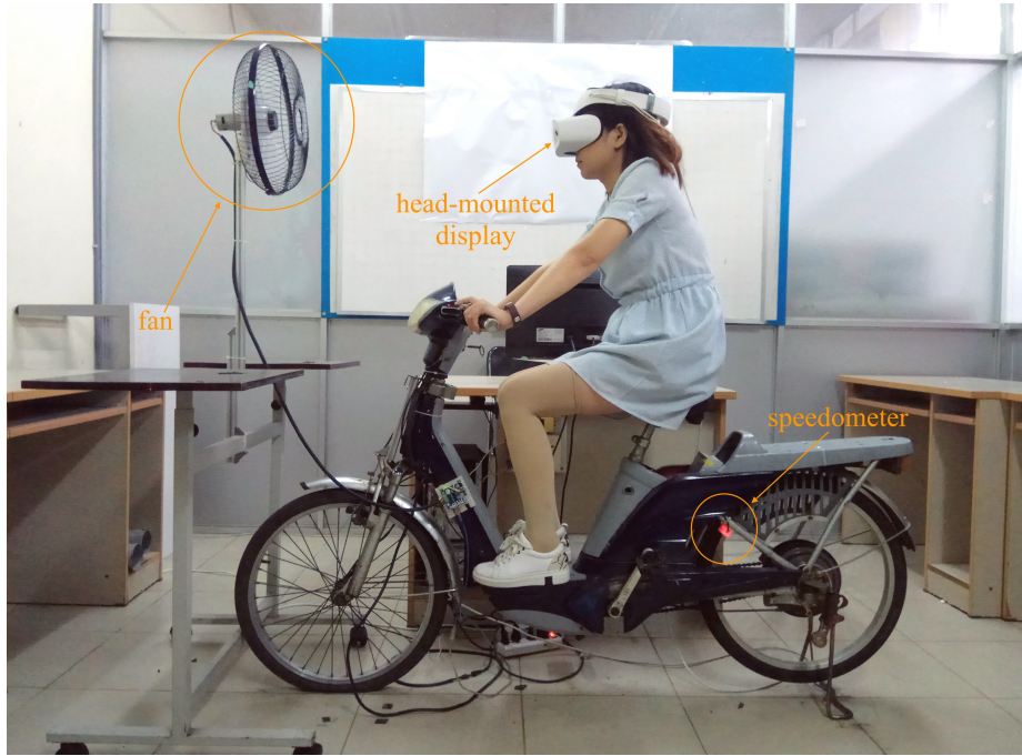
Fig. 1: Experiment Setup. Our experiment was conducted with a bike simulator. The simulator comprises of an electric bike with a head mounted display, a fan, and a speedometer.
