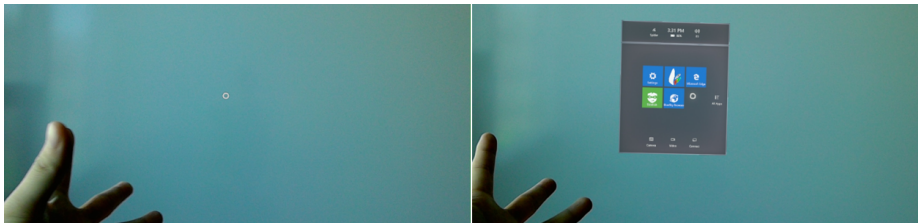
Fig. 4. Microsoft HoloLens can toggle between showing and hiding the main menu through a bloom gesture.
