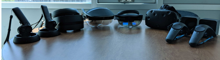
Fig. 5. Picture showcase a range of different HMD XR product. From left to right: HP windows mixed reality headset with inside-out tracked controllers, Meta 2 with built-in hand tracking, Microsoft HoloLens with gesture controls, HTV Vive with base station tracking. All these devices have differences that should be considered when designing for them.
