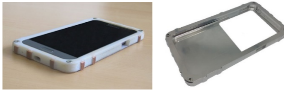
Fig. 4. : Two versions of the conductive case: a 3D printed version with copper strips (left) and a market-ready metallic version with strips already integrated on the edges (right). These were designed and engineered in collaboration with the technical college Renée Bonnet in Toulouse.
