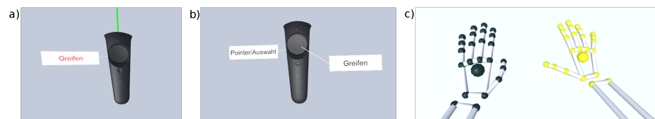
Fig. 1. Screenshots of HTC Vive based example implementations of three of our interaction modes: a) laser mode with controller attached tooltips, b) controller mode with tooltips, c) hand mode.
