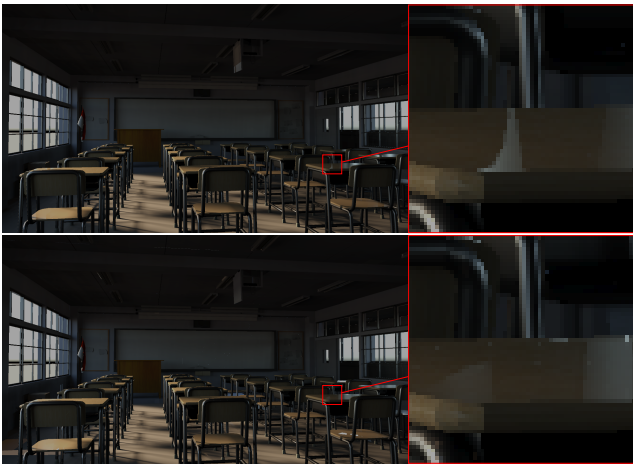
Figure 10: Poor refining caused by clustering not handling visibility can be enhanced by glossy surfaces, causing banding (top). Switching to a LightSlice alleviates this (bottom).
