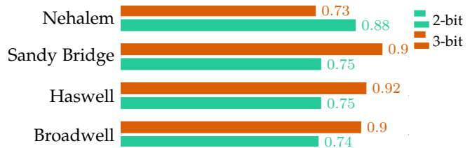
Fig. 1: Model accuracy on average for the 2-bit and 3-bit saturating counter state machines, for four micro-architectures.
