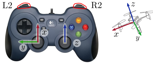
Fig. 10. Joypad used in conditions JN and JV. The left-hand thumbstick commands velocity along the x and y axes of the robot, while the right-hand thumbstick modifies its altitude. The two lower shoulder buttons R2 and L2 increases and decreases the external input \mu_\lambda(t) for the asymptote value of \lambda_2 , respectively.
