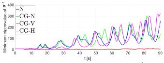
Fig. 7. Scenario #1. Evolution of the minimum eigenvalue of  ${\bf P}^{-1}$  (i.e., the maximum estimation uncertainty) for one representative subject in the four experimental conditions.
