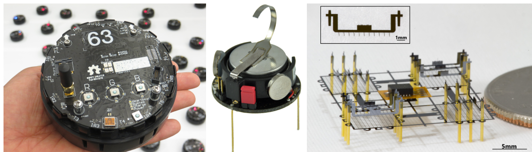
Figure 1: Robots used in swarm robotics come in different shapes and sizes: the dm -scale r-one [1] (left), the cm -scale kilobot [2] (center), the mm -scale ionocraft [3] (right).
