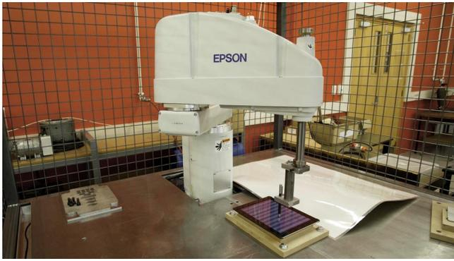
**Figure 5.** An an Epson G10-651S SCARA robot performing flicking gestures on an Apple iPad.
