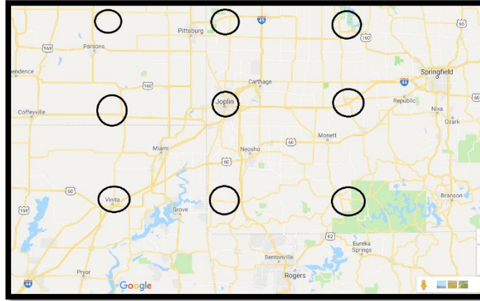
Fig. 2. Ideal positions of weather sensors for Joplin
