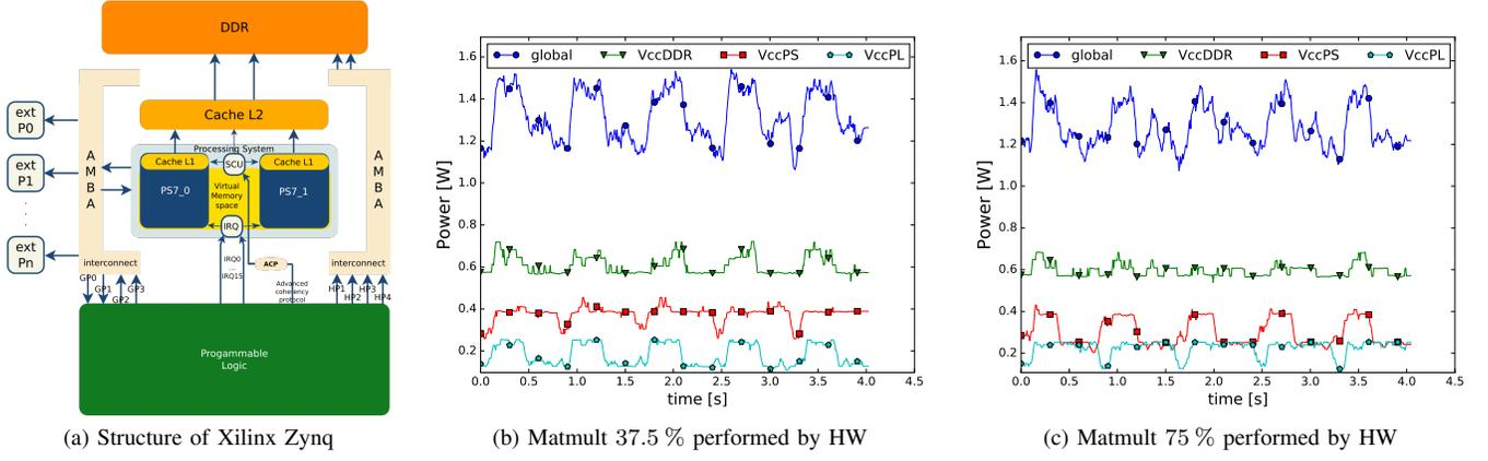
Fig. 5: Experimental infrastructure and power measurement traces.
