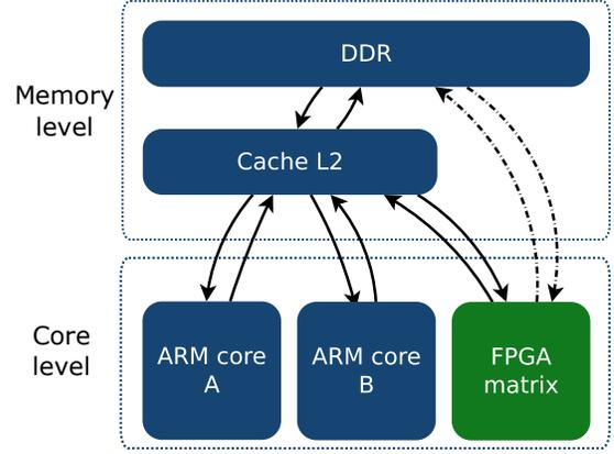
Fig. 3: Memory hierarchy of a Zynq architecture.
