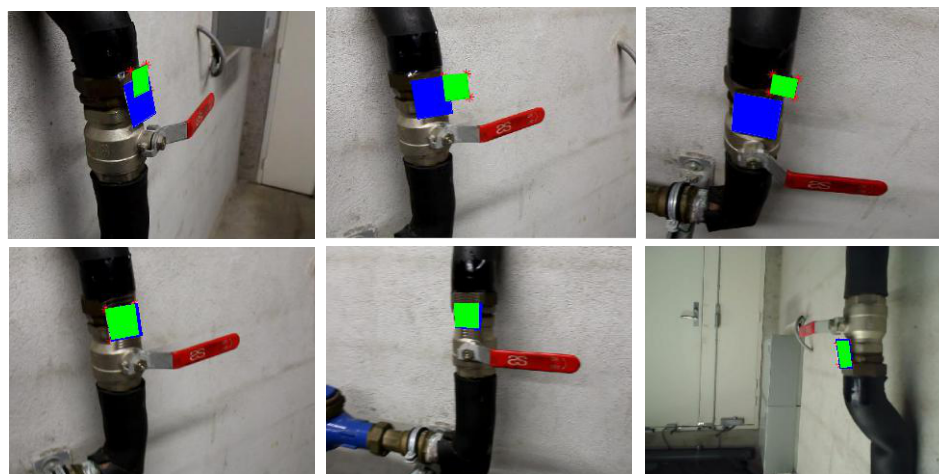
Figure 15. Comparison of marker reprojections (green) between the Industrial10-Traditional (upper) and Industrial10-WatchPose (lower) trained PoseNet. The ground truth is marked in blue.
