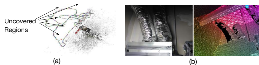
Figure 1. Challenges of collecting training data in industrial environments. (a) There are some uncovered regions within the training data using traditional video collection [6]. (b) There are some missing parts within the reconstructed 3D model on specular surfaces using Kinect Fusion [23,24].
