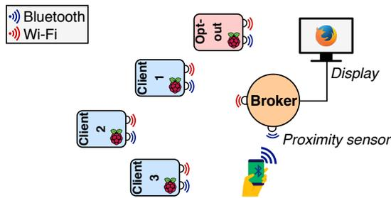
**Figure 1: Architecture of the *Venom* tracking system.**
